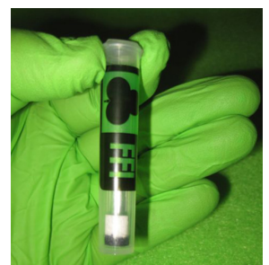
Example of chlorate positive, sampler tip turns from white to dark blue.
