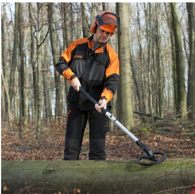
The fragment detector **EB 450 S** was designed especially for the forestry and timber industry. Its design is tubular and modular : all components of the device are integrated in a tube, which suppresses the need of cable links, thus improving product reliability. The battery compartment can be unscrewed to ease the transport.
