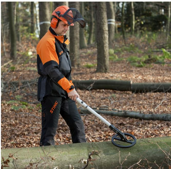
This device detects all conductive objects, ferrous and non ferrous metals, including small fragment or thin metal sheets. An audio alarm is given by an integrated piezo buzzer. A single rotary button is used to turn the device ON/OFF and to set the sensitivity.
