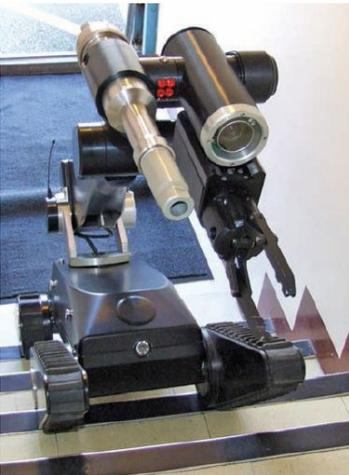
The GUARDIAN chassis has been developed to offer a highly stable and manoeuvrable platform. Track modules are able to move continuously through 360 degrees as independent front and rear pairs, ensuring great versatility in positioning, which in turn provides class leading obstacle negotiation capability and extremely stable stair climbing.
